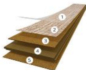
Figure 2. Cork floor panel structure 9
