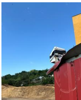
Figure 1. Measuring equipment for PM 2.5 and PM 10 on biomass storage
