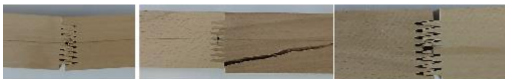
Figure 5. Characteristic joint failures
