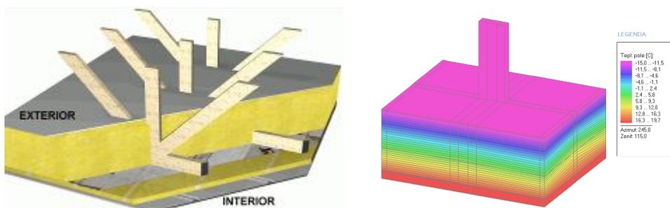
Figure 4. Ceiling composition and 3D thermal model with colour temperature distribution
