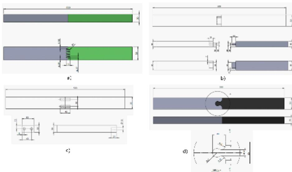
Figure 1. End-to end grain joints: a) finger joint, b) tenon joint, c) dowel joint, d) puzzle joint
