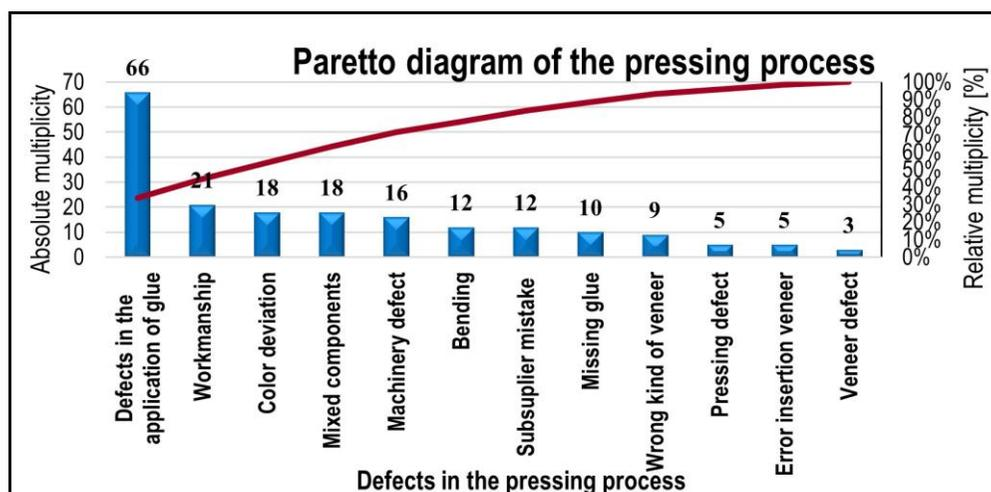
*Figure 3. Pareto diagram of the pressing process*
