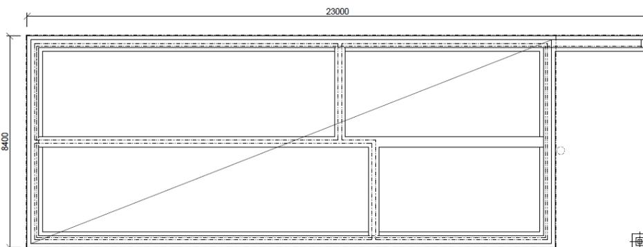
Figure 22: Floor plan of the foundation structures - the most used flat foundations.
