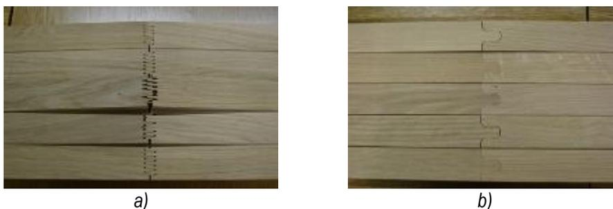
*Figure 5. Characteristic joint failures: a) finger joints, b) puzzle joints*
