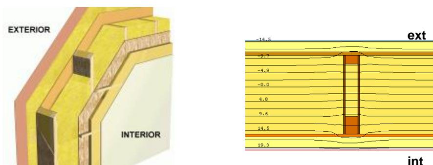
Figure 3. External wall composition and 2D thermal model with isotherms
