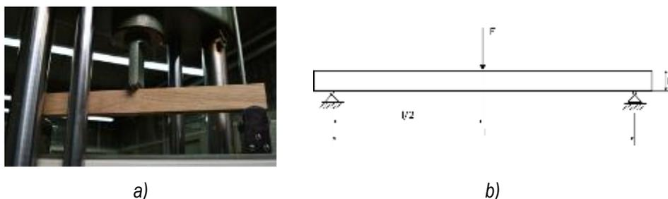
Figure 3. Three-point bending test: a) set-up of joint specimen in testing machine, b) diagram of loading
