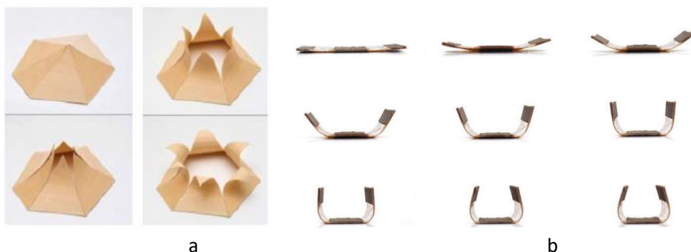
Figure 5. a - An example of a wooden structure based on a “wooden bimorph” [9]; b - A series of photographs in which a flat structure automatically transforms into a symmetrically curved structure, development of Self-Assembly Lab, MIT [3].
