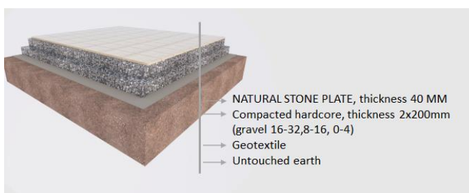
Figure 4. Structure of the natural stone plate terrace.
