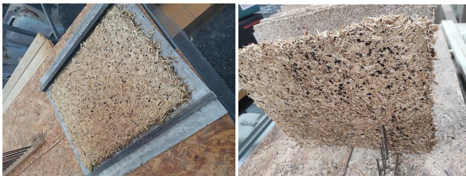
Figure 2. Woodrubber board (rubber ratio 10%) a Woodplastic board (pomer plastu lastic ration 15%)
