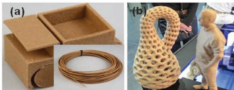
Figure 1. Developing lignocellulosic-based feedstock for 3D printing at FPIInnovations: (a) prototypes made using the powder-binding technology; (b) prototypes made using FDM technology (Li et al. 2016)
