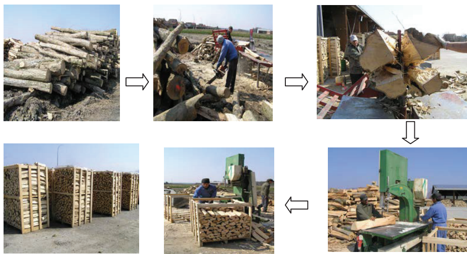
Figure 2. Overview of the production process of firewood following the arrows: the stack of the round wood longer than 1 metre in log yard; cross-cutting of round wood longer than one metre and production of one-metre round wood by a motor chainsaw; splitting one-metre round wood; cross-cutting of one-metre split wood with a band saw to the final length and additional splitting; disposing on pallets and air drying
