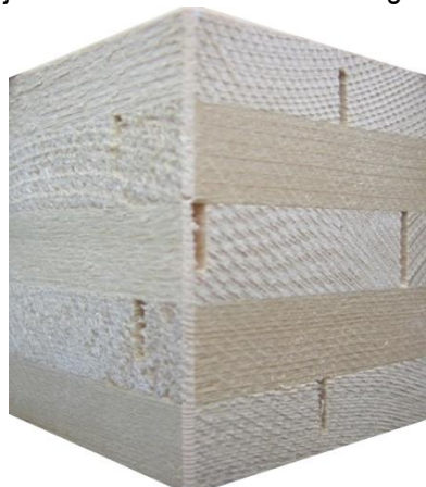
Picture 1. Five layer spruce CLT with grooves for stress reduction (Sretenovic P. 2014. Germany)
