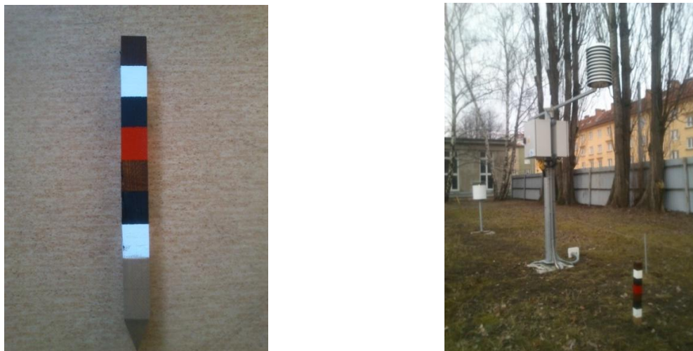
Fig 2 Wooden prism with protective coating (numbering from above) and Measuring site of meteorological station of University of Defense in Brno with planted wooden prism
