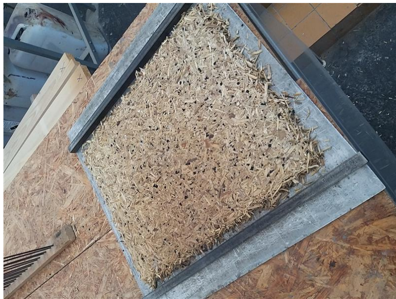
Woodrubber board (rubber ratio 10%)
