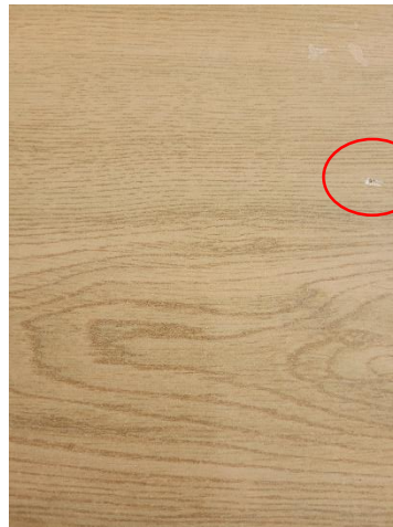
Level 2 – medium – small non-conformity in the right center
