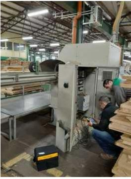
the electrical power was measured with Fluke 435-II Three Phase Power Quality and Energy Analyzers
