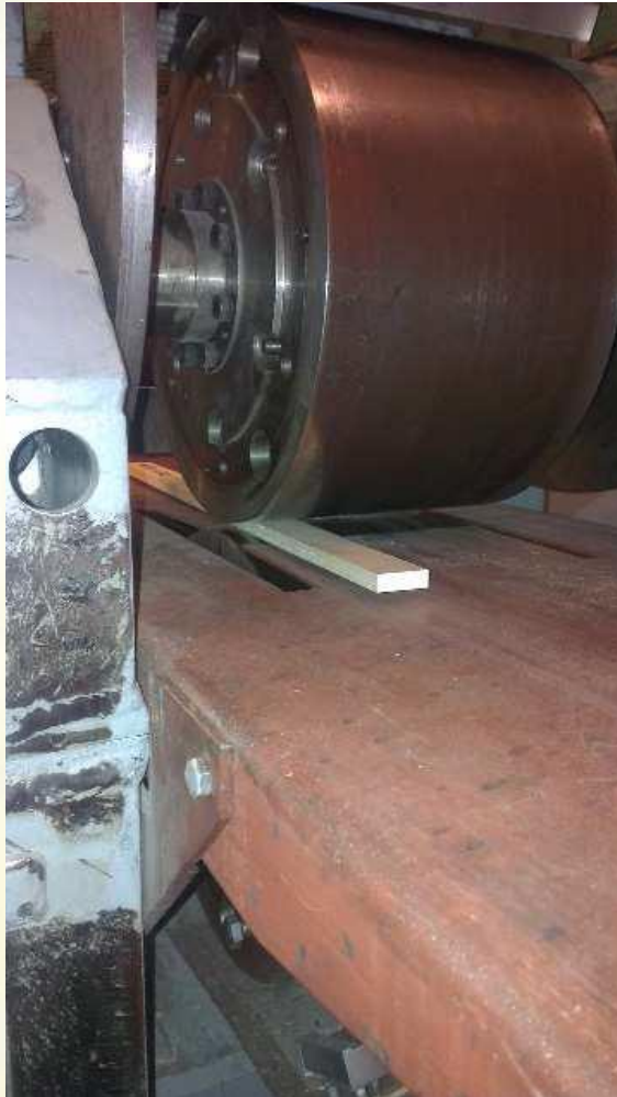
Fig. 2 Densification of wood by rolling
