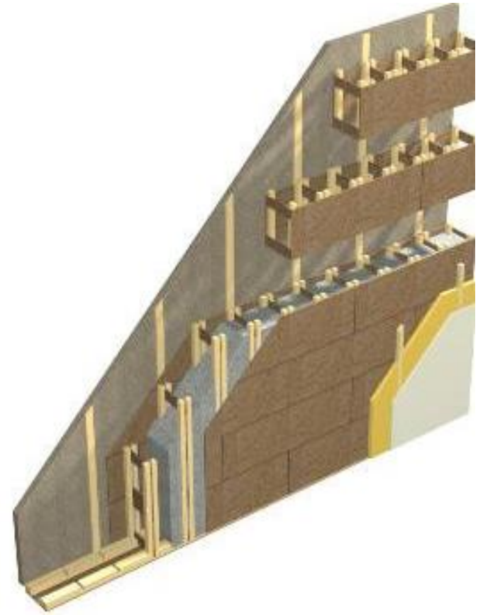
Wood frame light ladder construction thickness 34 cm
